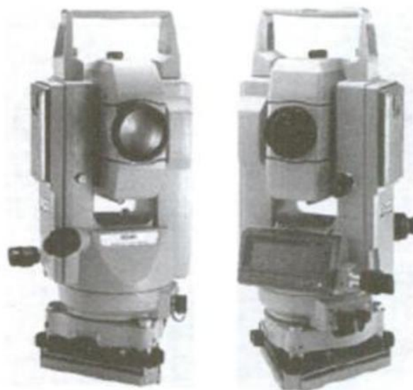
Figure 26.9 An electronic total station
