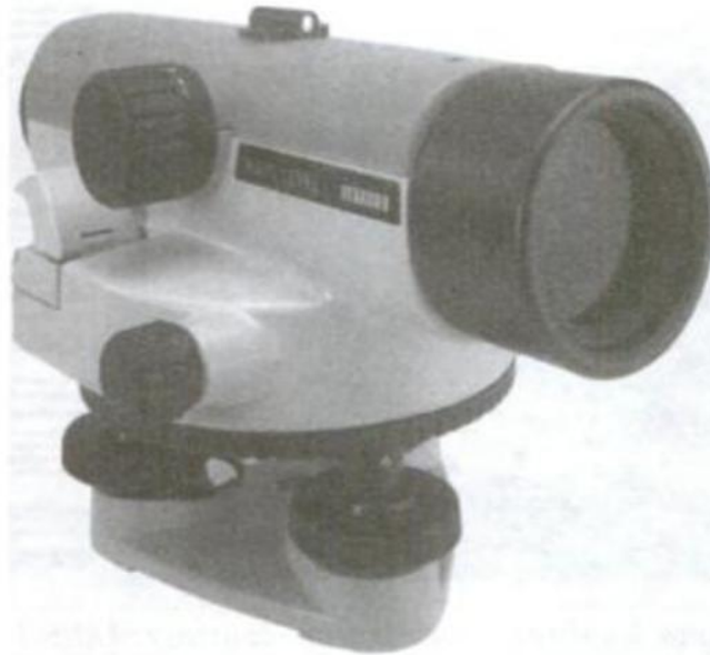
Figure 26.14 Automatic level (Pentax)
